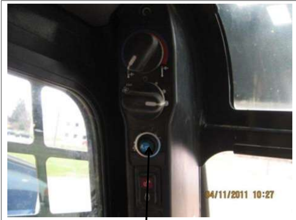
AC switch installed
