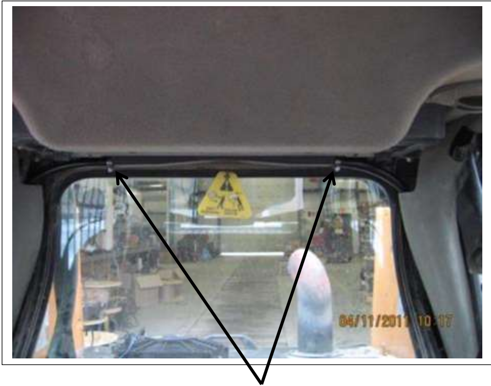
Connect drain tubes and feed as shown.
