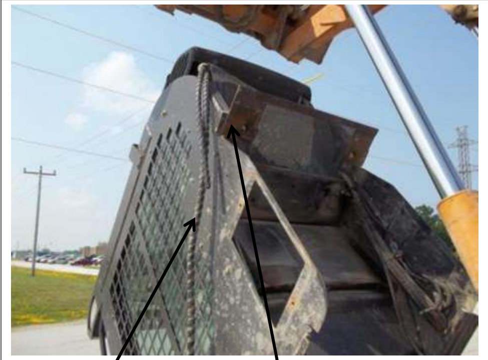
Hoses from evaporator wrapped with hose wrap.
