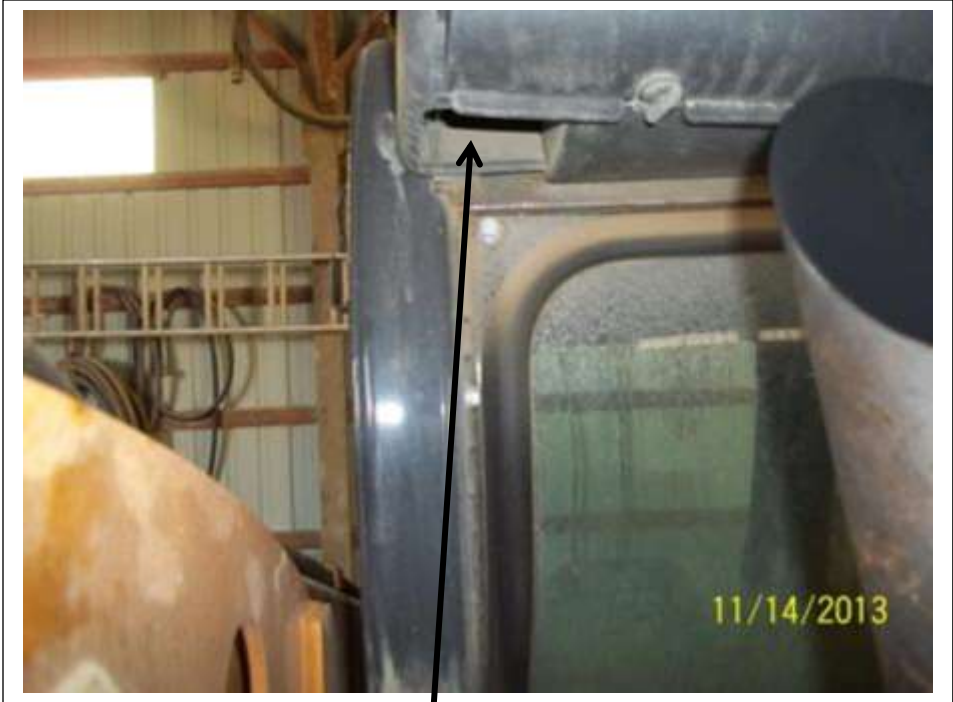
Hoses will come out here from evaporator
