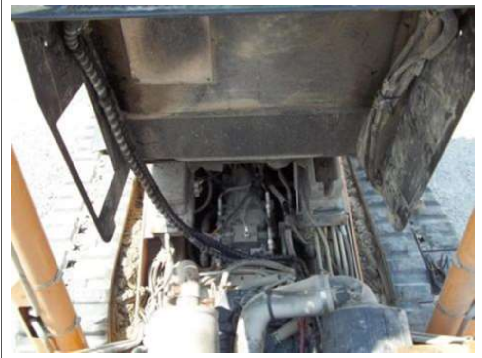
Fasten hoses such that they will not interfere with opening and closing of the engine compartment.
