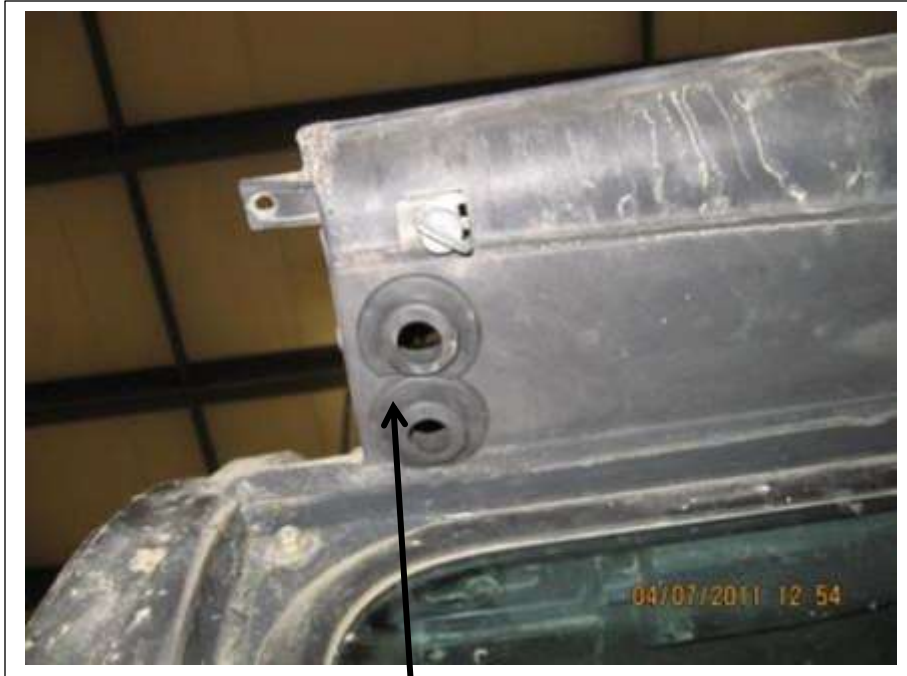
Two 1 1/8 holes drilled and grommets installed for the hoses coming from the evap.
