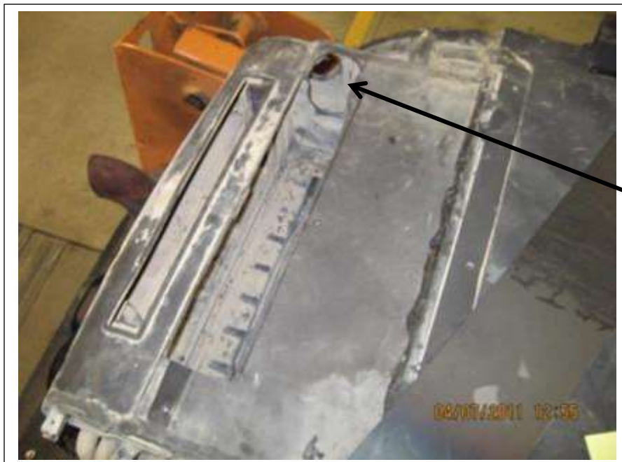
Clean out debris. Double check the cut out to ensure the fit for the evaporator coil.
