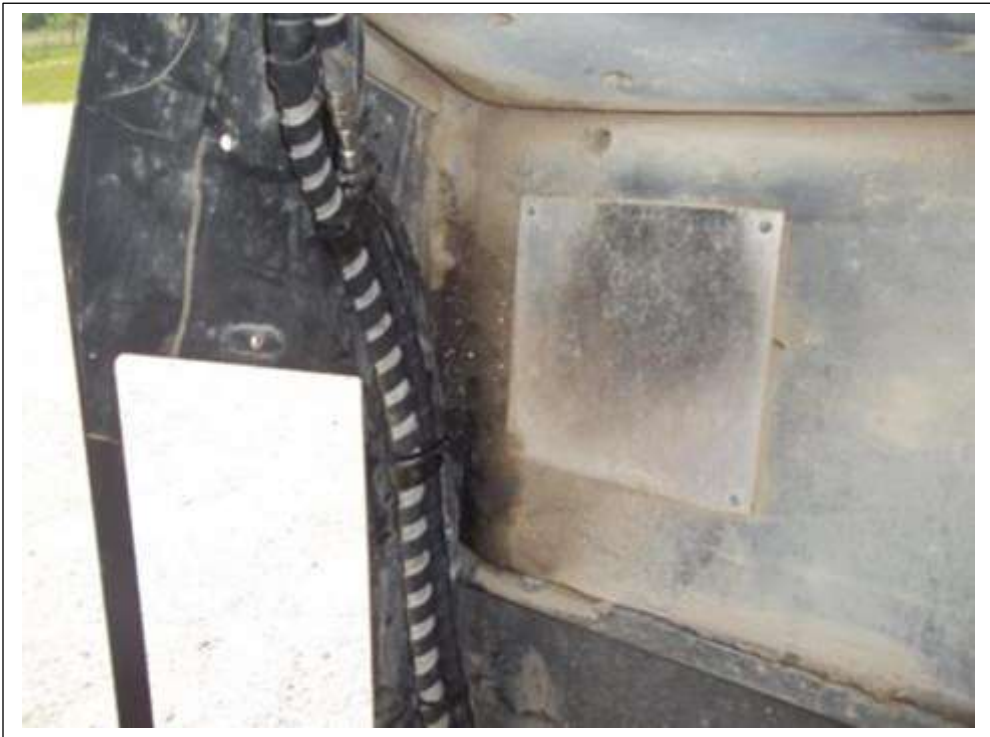
Fasten hoses such that they will not interfere with opening and closing of the engine compartment.
